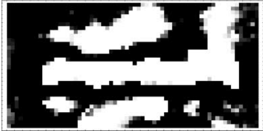
FIGURE 8 A map with a score of 552 out of a possible 578, created with a new learning method. While correctly declaring the hallway empty and walls occupied, it has overfitted to the data by declaring areas it can't sense as either occupied or empty instead of unknown. It could do this since the values it chooses for "unknown" areas don't affect the score.
