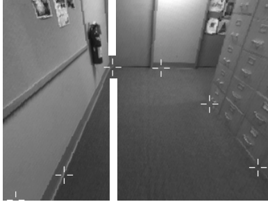
Figure 1: The vision subsystem semantics. Given a column in the image, the output of the evolved program was interpreted as the boundary between ground (lower white line) and the lowest non-ground (upper white line). Show is the ground truth in six different columns.
